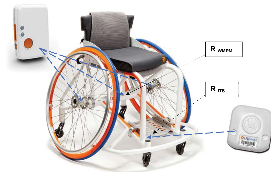
Figure 1: Wheelchair measurement setup, with the Ubisense tag (ITS) mounted on the footplate and the Shimmer3 inertial sensors on frame and wheels. The reference point for the ITS ( R_{ITS} ) is the same as the tag, whereas the reference point for the WMPM ( R_{WMPM} ) is the frame centre.
