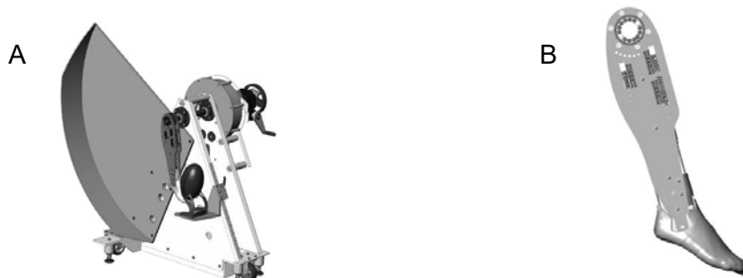
Figure 1. The kicking machine (A) and limb with spring mechanism (B).
