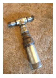
Figure 2 Soil Sampling Tool
