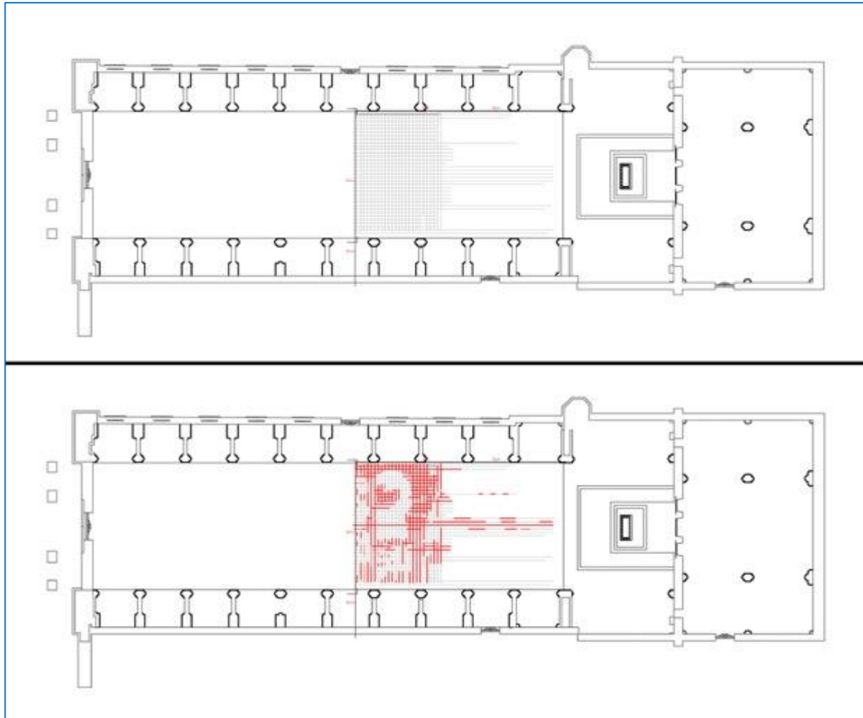
Figure 10 Santa Chiara, Naples, church plan showing the GPR data acquisition paths (above) and the subsurface materials recorded by the GPR instrument (below), courtesy of Leopoldo Repola. Photo: author.
