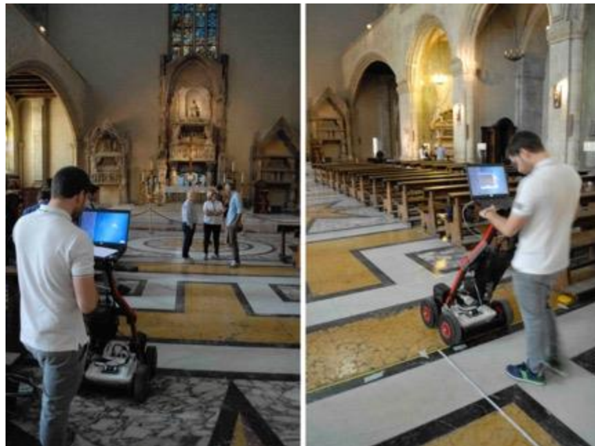
Figure 9 Santa Chiara, Naples, ground-penetrating radar process. Photo: author.
