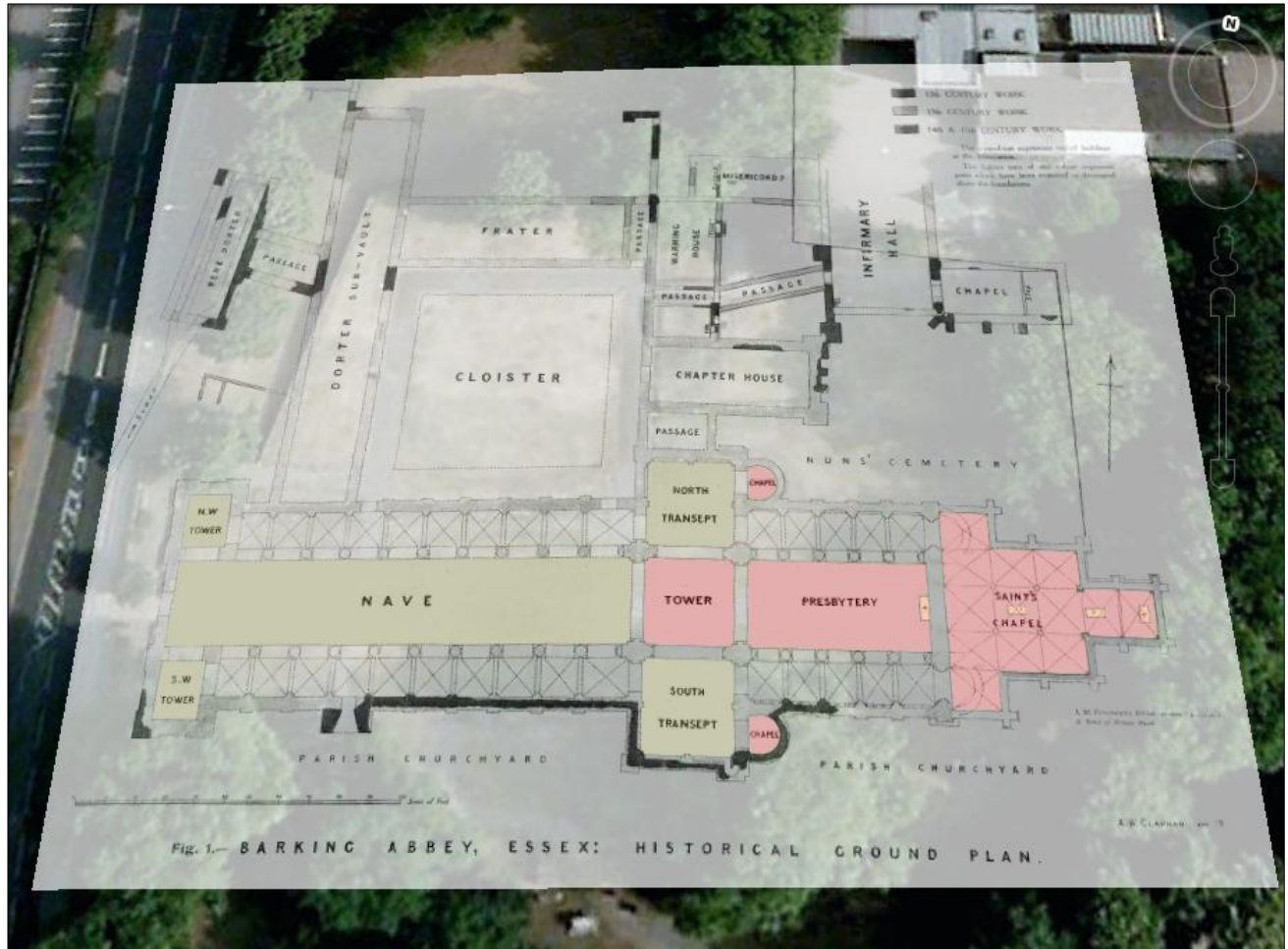
Figure 4 Digitizing polygons of the internal Abbey church structures using the Clapham image as a reference
