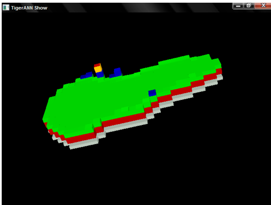
Figure 16. 3D Surfer- Pressure distribution-layer No.1. (Connected cells).
