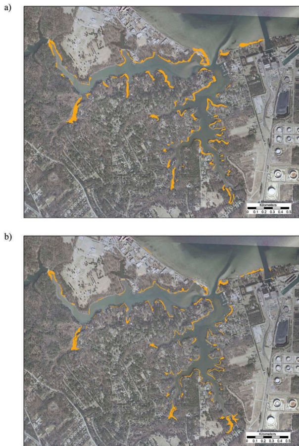
Figure 4. Wormley Creek, York VA. Example of marsh fragmentation and loss due to shoreline stabilization. (a) Old TMI marsh distribution shown on an aerial photo from 2009. (b) New TMI marsh distribution shown on an aerial photo from 2009.
