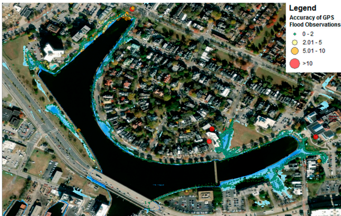
Figure 10. Map of radial positional accuracy (in meters) reported by the Sea Level Rise mobile app in Norfolk's Hague during Catch the King 2017. Points in red were not included in the spatial comparison.
