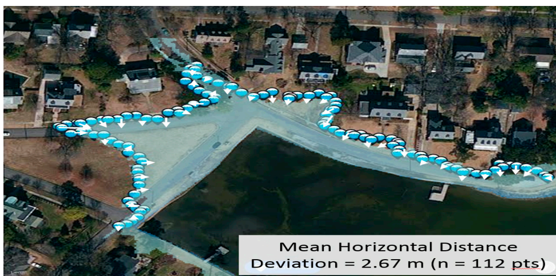
Figure 7. Illustrative comparison of mean distance difference of 112 GPS data points collected in Larchmont, Norfolk (2.67 m), compared with the 2018 king tide peak inundation forecast in blue.
