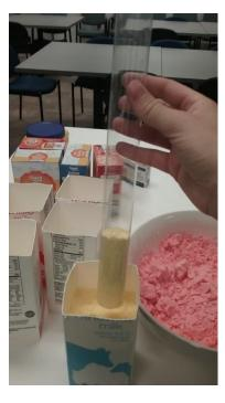
The next page is an example of how I fill the cartons with sediments. First I mark an inside edge with a ruler and pen. Each mark shows the top height of each layer above the layer below it. Then I slowly add mixture and pack it down layer by layer. This example shown below is for a core from a different lesson plan, which is outlined as follows:
