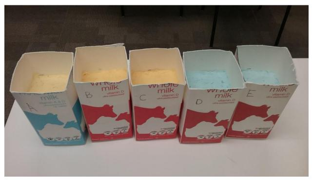
Example of finished bins prepped for a lesson plan using quart milk cartons. I cut each carton to be 15 centimeters tall. I cut the coring tubs (fluorescent light bulb protectors) to be about 30 cm in length so the students had plenty to grip while coring (below).
