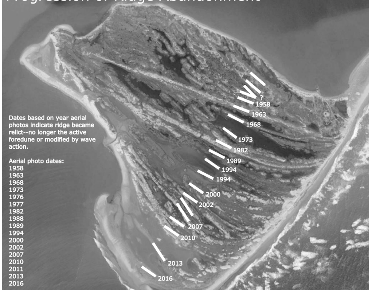
Figure S5. Aerial photo of Fishing Point showing progression of dune ridge abandonment along the cross-shore transect through time. 2013 image selected as base due to high resolution and contrast. Map data: Google, USDA Farm Service Agency.
