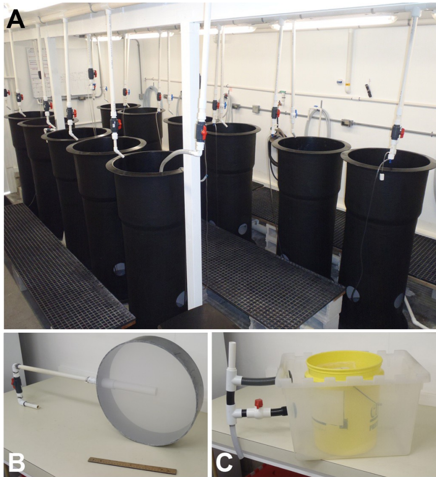
Fig. 4. An example large scale culturing set up. A) Interior of climate controlled larval rearing room. The black cylinders are 200-L cone bottom larval rearing tanks where larvae and phytoplankton are suspended with gentle aeration. B) Banjo screens are used for daily water exchanges by reverse filtration; this is a larger version of the reverse filtration apparatus shown in Fig 1A. C) When larvae need to be moved, or if the tanks are in need of thorough cleaning, forward filtration is carried out using a screened bucket and tote system as described in the legend to Fig. 3. The principle is the same as the set-up shown in Fig. 2, but at a larger scale. Photos by D.L. Cohen.
