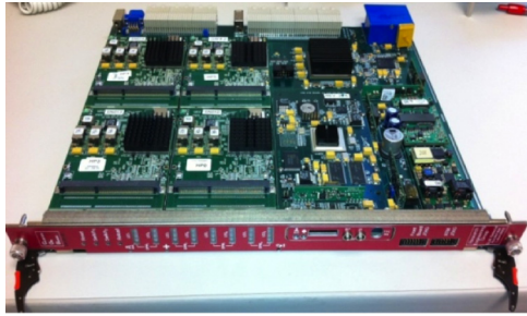
Fig. 9. The SVT DAQ COB board with four data processing daughter cards (DPMs) visible on the left side.
