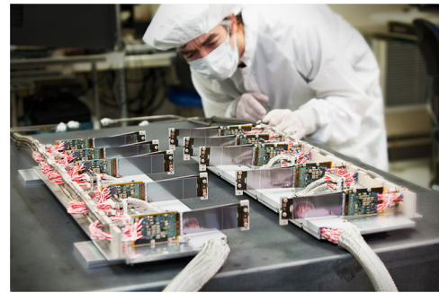
Fig. 4. Both halves of the HPS Test Run SVT after final assembly at SLAC. The cooling manifolds and integrated cable runs are clearly seen.
