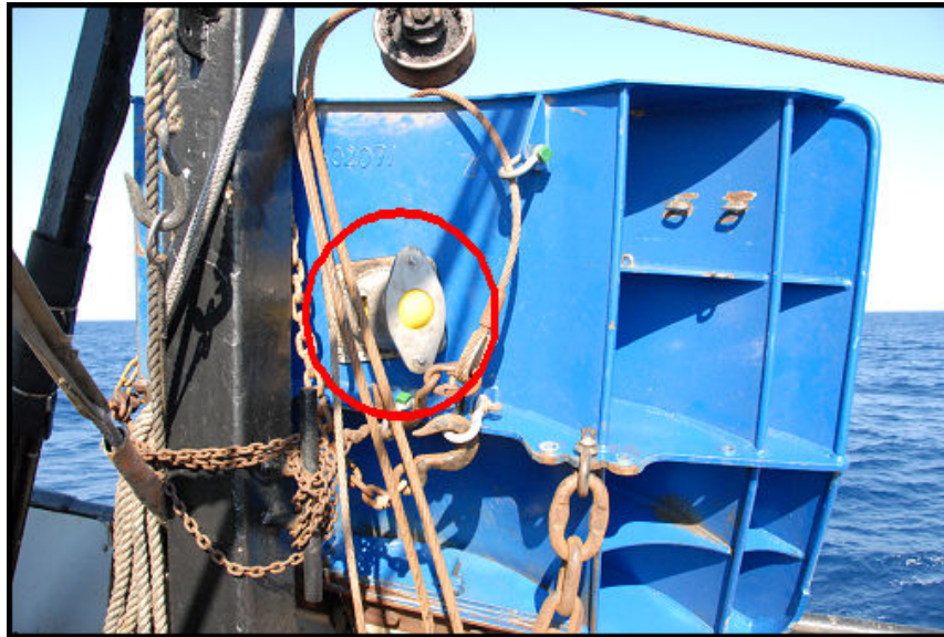
Figure 2. Thyboron Type IV 66" trawl doors frontside (A) and backside (B) with mounting bracket for Netmind sensor.
