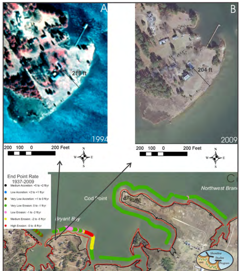
Figure 2-7. Determining rate of change along the shoreline. Aerial photos of a site in Gloucester County in A) 1994 and B) 2009. C) The end point rate of shoreline change determined between 1937 and 2009. Rates are visualized as different colored dots and show the variability of rates of change along small sections of shore (from Milligan et al. , 2010).
