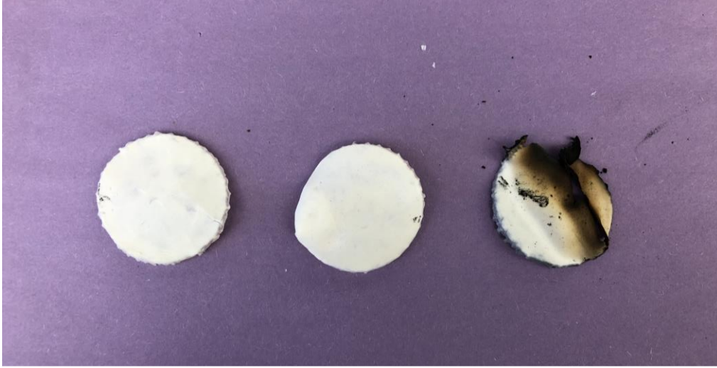
Figure 10: Flame tested ABS samples with 15% Mg(OH) 2 by weight. From left to right: 1 second of thermal exposure, 3 seconds of thermal exposure, and 5 seconds of thermal exposure.
