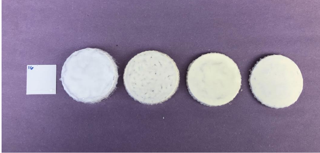
Figure 4: ABS samples studied. From left to right: 3D printed ABS filament, ABS cast from acetone, ABS with 3% \text{Mg}(\text{OH})_2 by weight, ABS with 9% \text{Mg}(\text{OH})_2 by weight, ABS with 15% \text{Mg}(\text{OH})_2 by weight.
