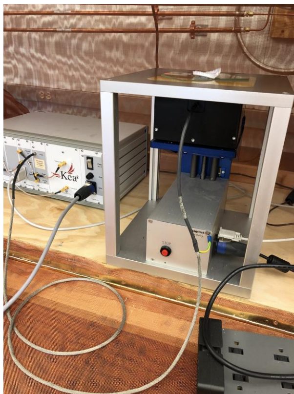
Figure 3: The PM5 in the mechanical lift and the Kea2 spectrometer with an ABS sample atop the sensitive region on the magnet. For deformed samples, glass slides were used to stabilize the sample, keeping the sample flush with the sensitive region for the duration of the T_2 experiment.
