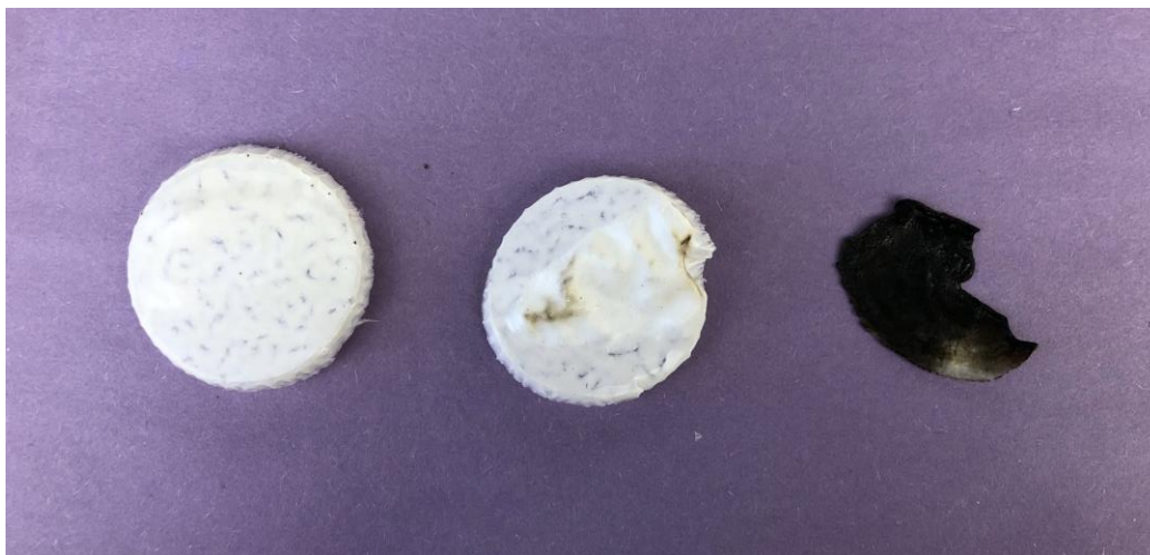
Figure 8: Flame tested ABS samples with 3% Mg(OH) 2 by weight. From left to right: 1 second of thermal exposure, 3 seconds of thermal exposure, and 5 seconds of thermal exposure.
