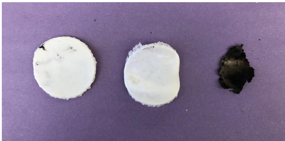
Figure 9: Flame tested ABS samples with 9% Mg(OH) 2 by weight. From left to right: 1 second of thermal exposure, 3 seconds of thermal exposure, and 5 seconds of thermal exposure.
