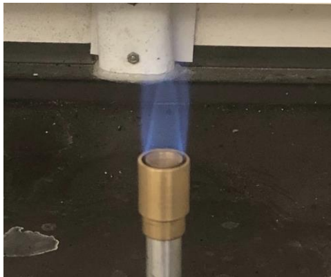
Figure 5: Bunsen burner flame set up as outlined in the test methods section of NFPA 1971. 1 The inner cone is about 25 mm in height and the outer cone is approximately 50 mm in height. The resultant flame is approximately 1200°C.
