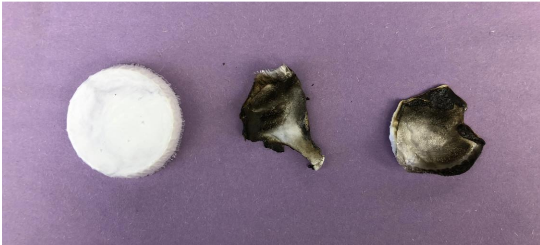
Figure 7: Flame tested ABS samples cast from acetone. From left to right: 1 second of thermal exposure, 3 seconds of thermal exposure, and 5 seconds of thermal exposure.
