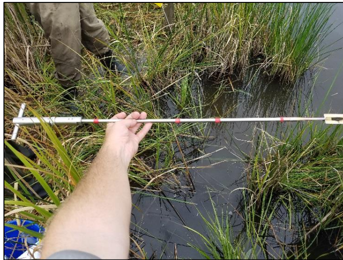
Figure 3 – Humboldt Shear Vane with various measurement depths taped in red. Handle gauge to left of hand in photo.
