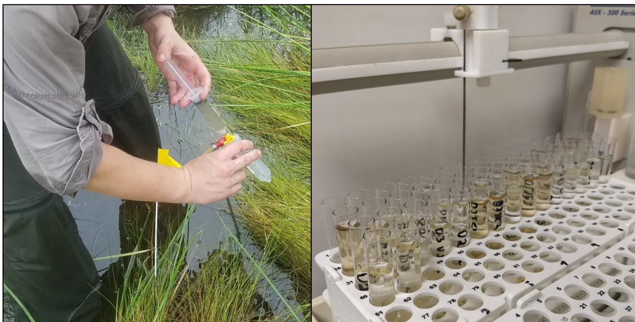
Figure 4 – (Left) Extracted porewater filtering through 45-micron filter and stored in 50mL tube for later Ammonium testing. Porewater used for sulfide levels was stored in smaller prepared scintillation vials. (Right) Water samples being sent to Lachat analyzer post spiking and sparging.
