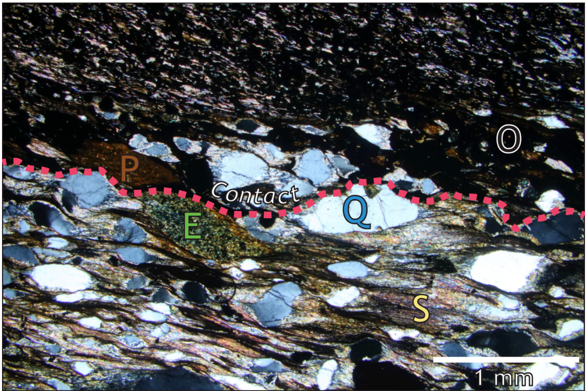
Figure 35b. Localized area of opaque (O) mineral concentration. Epidote (E) grains are elongated, and halos of sericite (S) surround the quartz (Q) grains. The beginnings of pressure shadows appear around the quartz, as well, and there is a contact with the more plagioclase-rich fine-grained purple phyllite.
