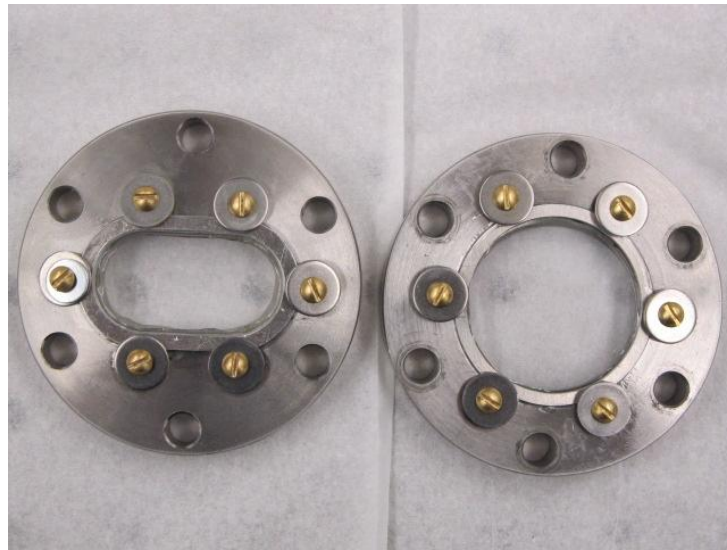
Figure 5: Left, the polypropylene window. Right, the KBr window.
