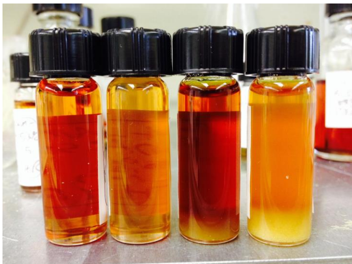
Figure 14: Polymer Solutions From Left to Right: UDA-BAM, UDA-BAM-BTDA-17% THERM, UDA-BAM-BTDA-25% THERM, UDA-BAM-BTDA-33%THERM
