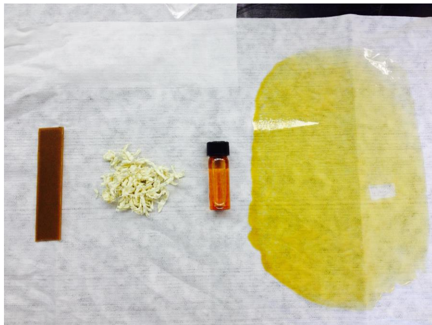
Figure 8: Polymer Products - From Left to Right - Pressed Block, Polymer Flakes, Liquid Sample, Film
