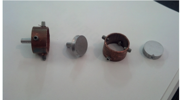
Figure 22: Modified sample tabs for imaging with both SEM and AFM. The assembled tab is on the left, and the disassembled components are on the right.
