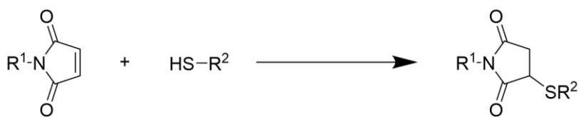
Scheme 1. General Reaction for Addition of a Thiol across a Maleimide Double Bond
