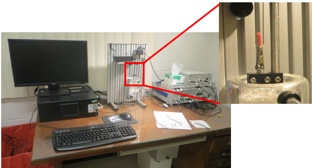
Figure 3. Aurora Scientific Instruments Model 807B in situ large rodent/small animal apparatus that was used to stimulate and measure the contractile force. The inset shows a muscle on the apparatus.
