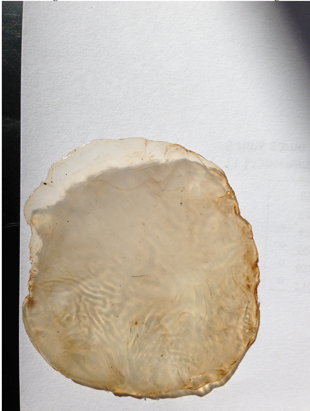
Figure 3.1.1.3: 20130919 Neat PA-11 Film After Pressing
