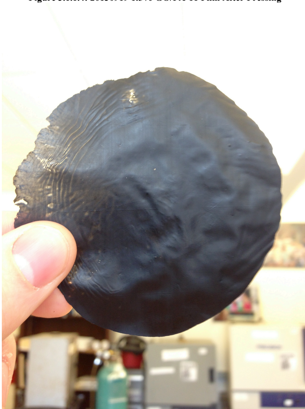
Figure 3.1.1.4: 20130919 1.5% GO/PA-11 Film After Pressing
