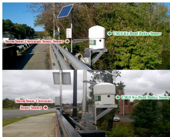
Figure 5. Examples from three StormSense ultrasonic sonar sensors co-located in the field adjacent to USGS K a -Band radar sensors in Virginia Beach for direct comparison of monitoring accuracy. These sensors will temporarily be stationed adjacent to each other for a period of 6-9 months to provide a long term data record for comparison of water level measurements, data transmission speeds, and solar power efficiency. Figure adapted from [4].
