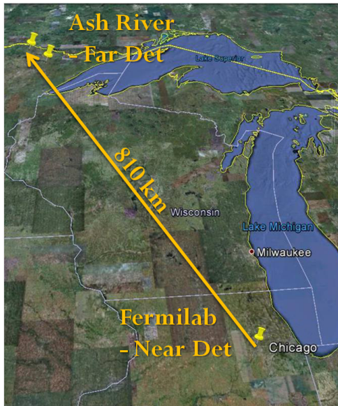
Figure 1. The NO \nu A Far detector is located at a site in Ash River, MN which is 810 km from Fermilab at an angle of 14 mrad of the primary NuMI beam axis. This puts the NO \nu A detector at an L/E corresponding to the first oscillation maxima. The 14-kton Far Detector (FD) is currently under construction and The 0.3-kton Near Detector (ND) will be located on the Fermilab site in a new cavern, excavated near the existing MINOS Near Detector Hall. Also, the construction of Near detector has already started.
