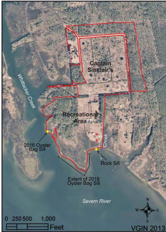
Figure 2-4. Location of shore protection structures at Captain Sinclair's Recreational Area.
