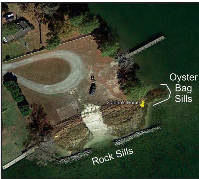
Figure 4-13. Location of oyster bag sill at Site 3, St. Johns Point on Free School Creek.
