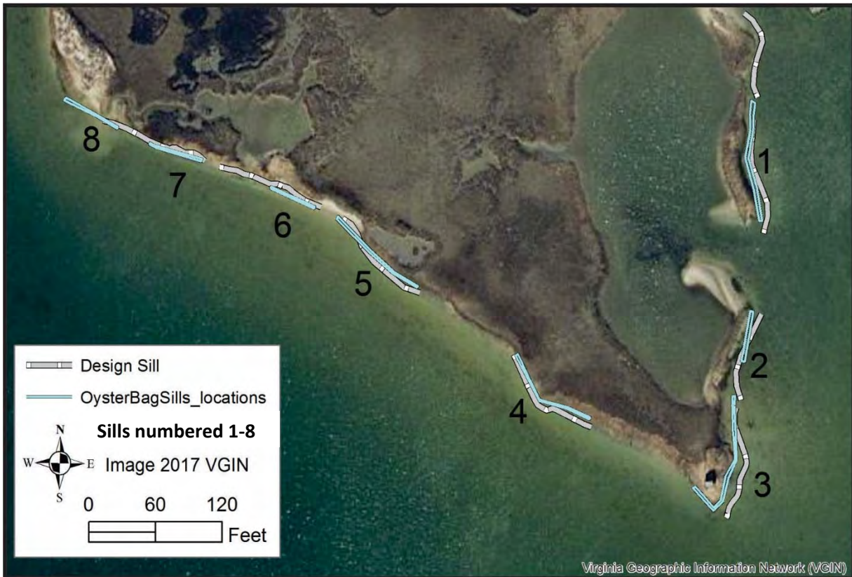
Figure 5-8. Comparison between the location of the oyster bags sills (numbered 1-8) in the design (white) and what was installed (blue).
