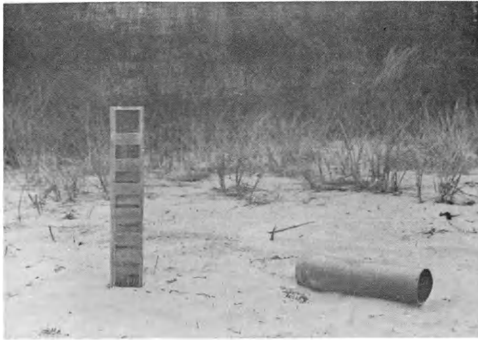
Figure 52. Sand trap and portable anemometers used to measure eolian sand transport. Section of PVC pipe (bottom) was used to dig a hole for placement of sand trap.
