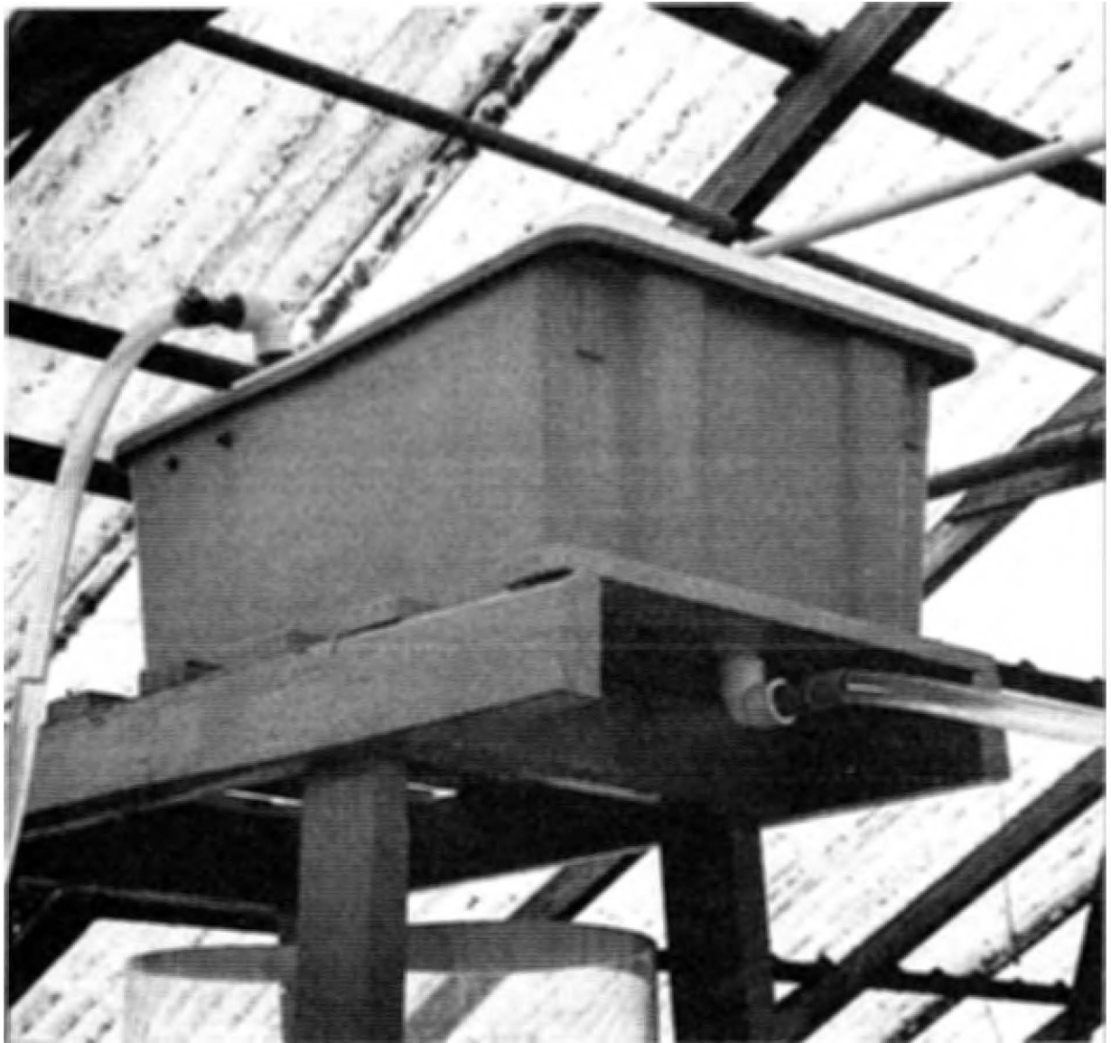
Head tank for washdown table showing location of thru-hull fitting (right) and intake tubing (left). Ref. p. 74.
