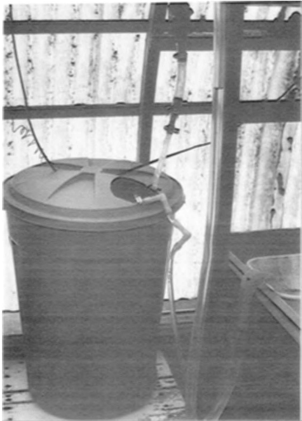
Heat exchanger, external view, showing thermostate wire (coil) leading in from left, water control valve at top right and drain into spawning trough at right. Ref. pp. 9 - 14.
