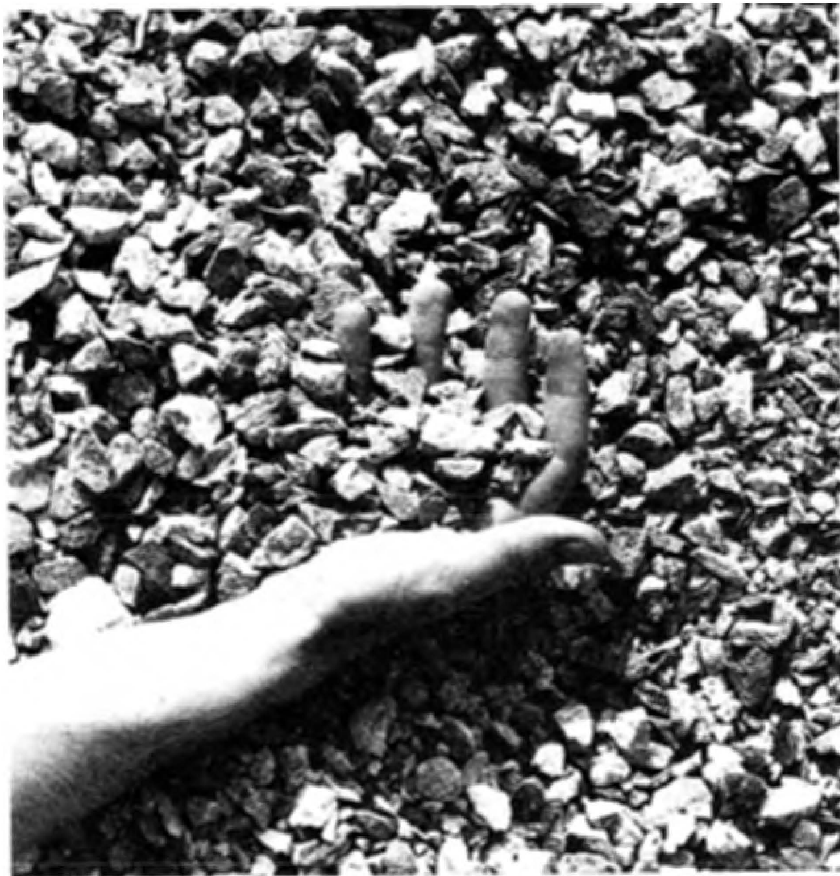
Note size and angularity of aggregate for planting beds. No. 8 crushed stone, shown here, is the preferred material. Ref. pp. 41 - 42.
