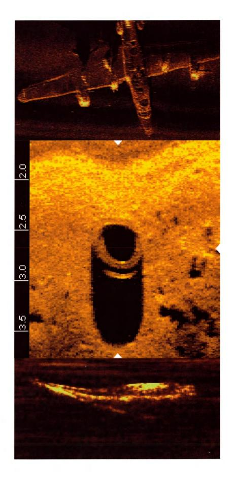
**Figure 2.** A. Sample output of a digital sidescan mosaic, gathered by an AUV at 2.2 kt (1.1 m/s) in depth-following mode (2.5 m depth, water column 5.5 m deep). B. Navigation track lines interpolated by the mosaicking software, Sonar Web Pro (Chesapeake Technology). C. Geo-reference mosaic shown on aerial photo of the York River, Virginia (37° 13.61' North, 76° 29.25' West), where these data were gathered.
