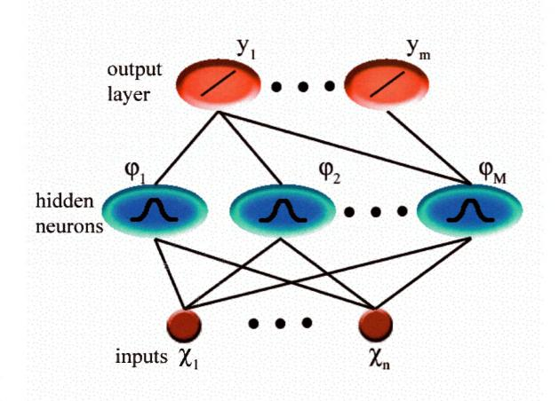
**Figure 6.** Schematic diagram of the image classification approach used in this study. Features (components of the image vector) are extracted from the raw sidescan sonar images and input to the RBF neural net classifier. The RBF architecture allows the classifier to be easily scaled up to classify new species as ground-truthed data become available.
