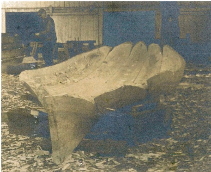
Figure 4. Keel log, garboard and additional logs form a five log canoe at Darlings Railway, Circa 1937. Courtesy of the Hampton History Museum, Hampton, Va., 2008.63.14, Detail.
