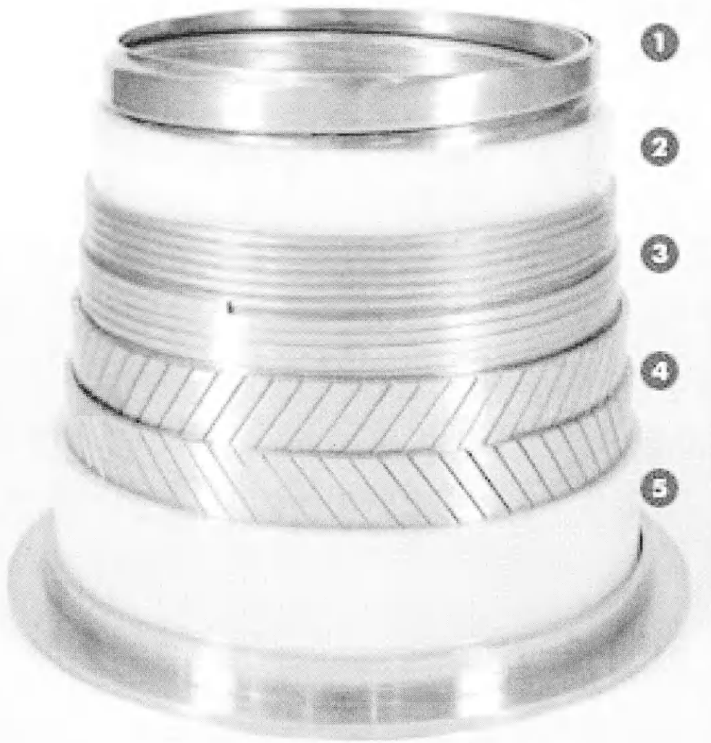
Figures 1.1: Construction of NKT Flexibles' PA-11 pipe. Layer 1 is made of steel. Layer 2 is the PA-11 liner. Layers 3 and 4 are made of steel tape. Layer 5 is an outer rubbery layer. [8]
