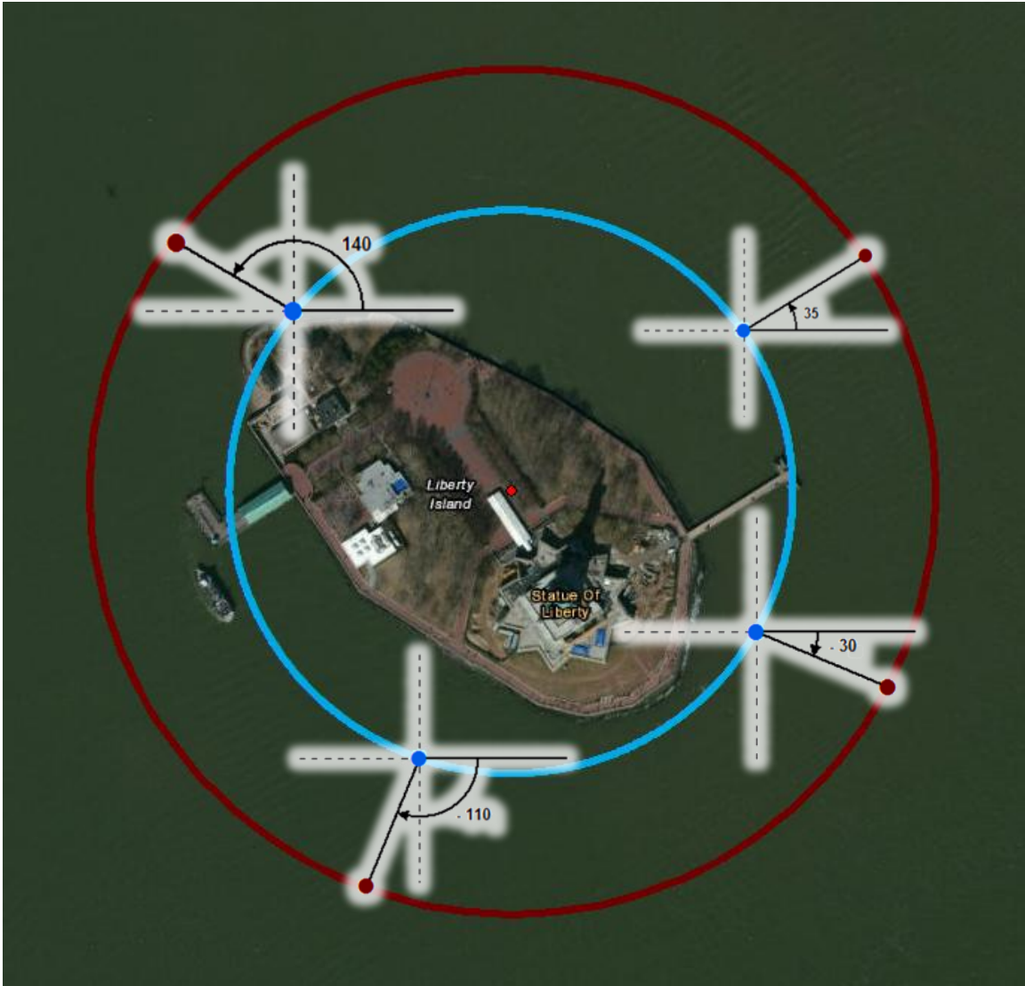
Figure 5.5. Ideal test case for distance measurements showing two concentric circles with radii of 200m (in blue) and 300m (in red). The blue circle is comprised of 1256 points evenly spaced 1m apart, with the nearest distances from each blue point to the outer red circle and resulting angles calculated relative to 0° at due east outputting to a GIS table.
