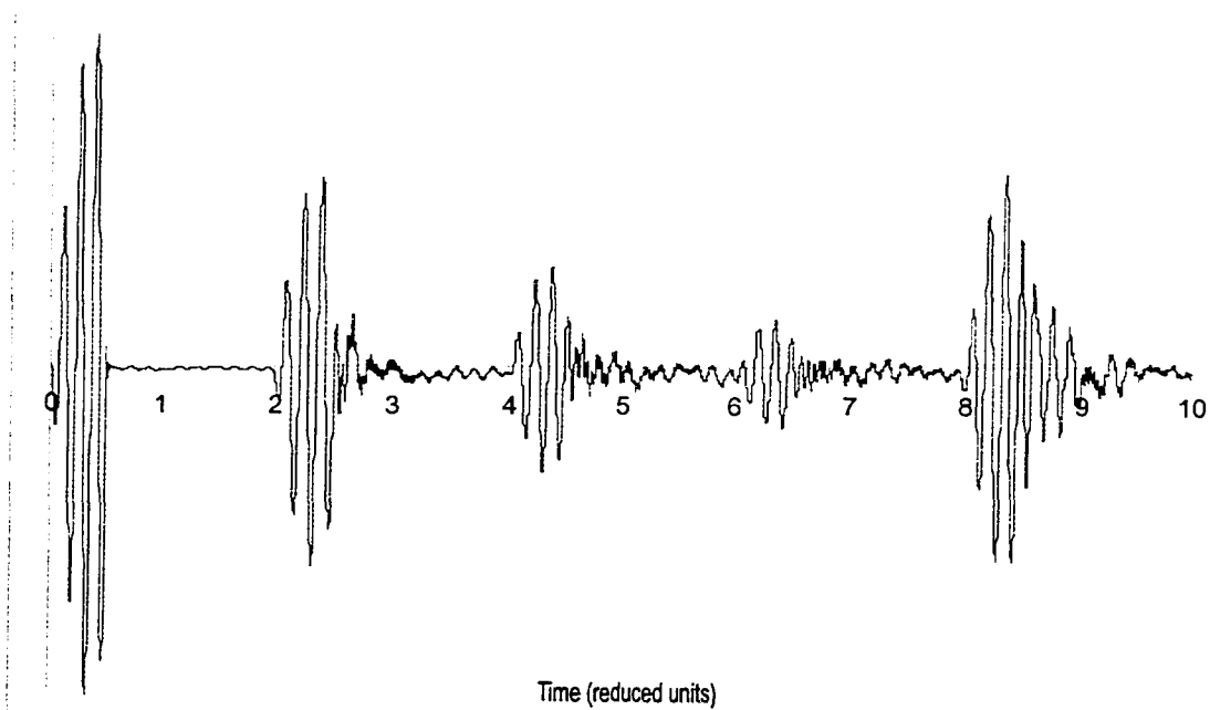
Figure 7.8: Trace for simulation with a surface irregularity at 1 r.u. (distance).
