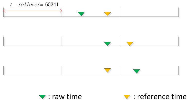
FIG. 3.4: Three possible cases are shown here. In the top diagram, the raw drift-time and reference time appear in the same time window, so the direct subtraction is sufficient; for the middle diagram, the reference time and raw drift-time are in different window, so in order to calculate their difference, an offset must be added to reference time, thus: \Delta t = t_{reference} + t_{rollover} - t_{raw} ; for the bottom diagram, similar to the second case, the offset must be added to the raw drift-time in order to get the right difference: \Delta t = t_{raw} + t_{rollover} - t_{reference} .
