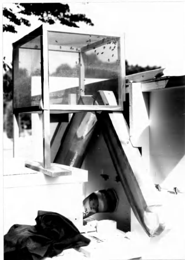
FIGURE 5: (right) Photograph of collecting cage and funnels at back of apparatus.
