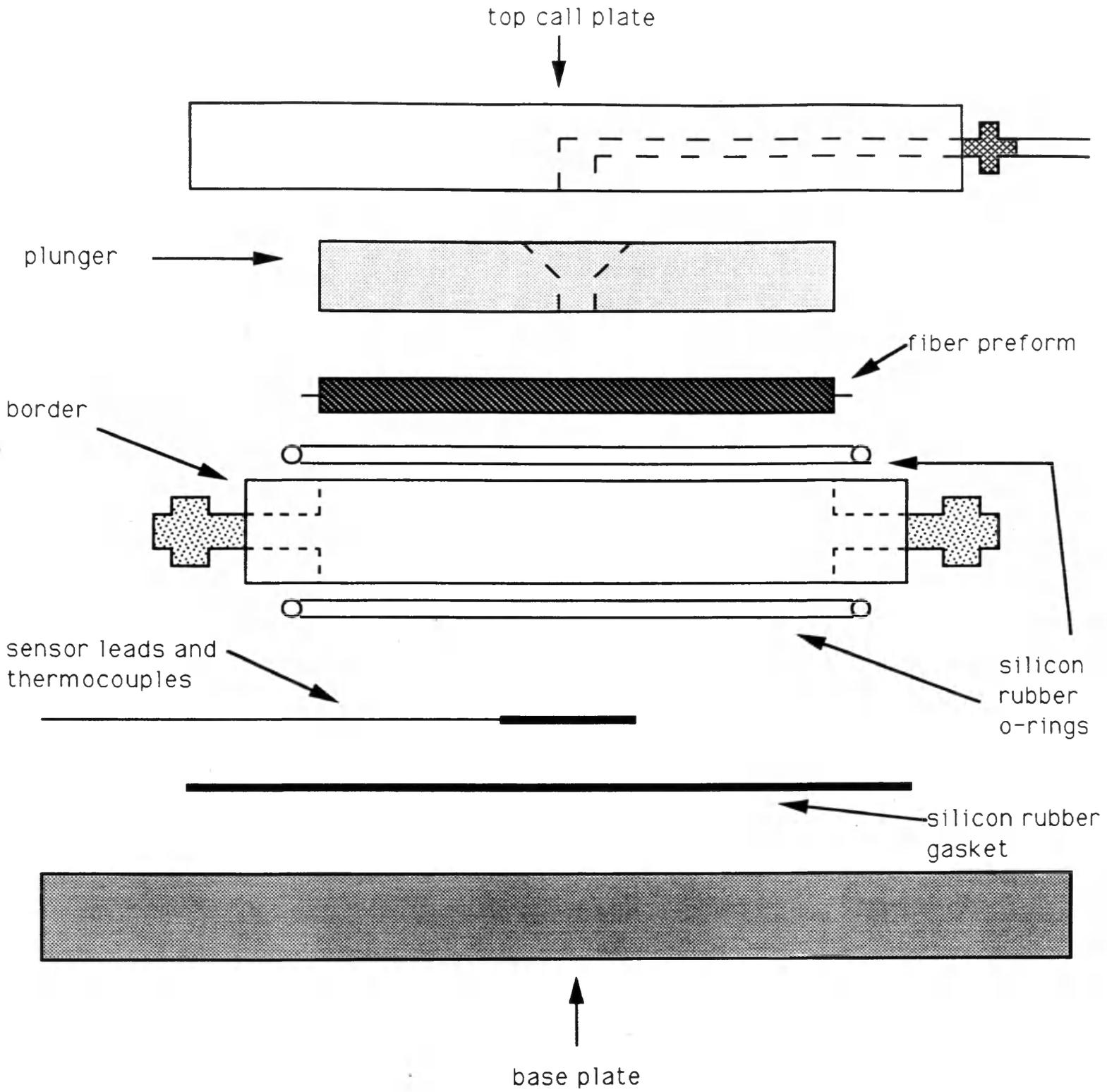
Schematic of Mold Lay-up
