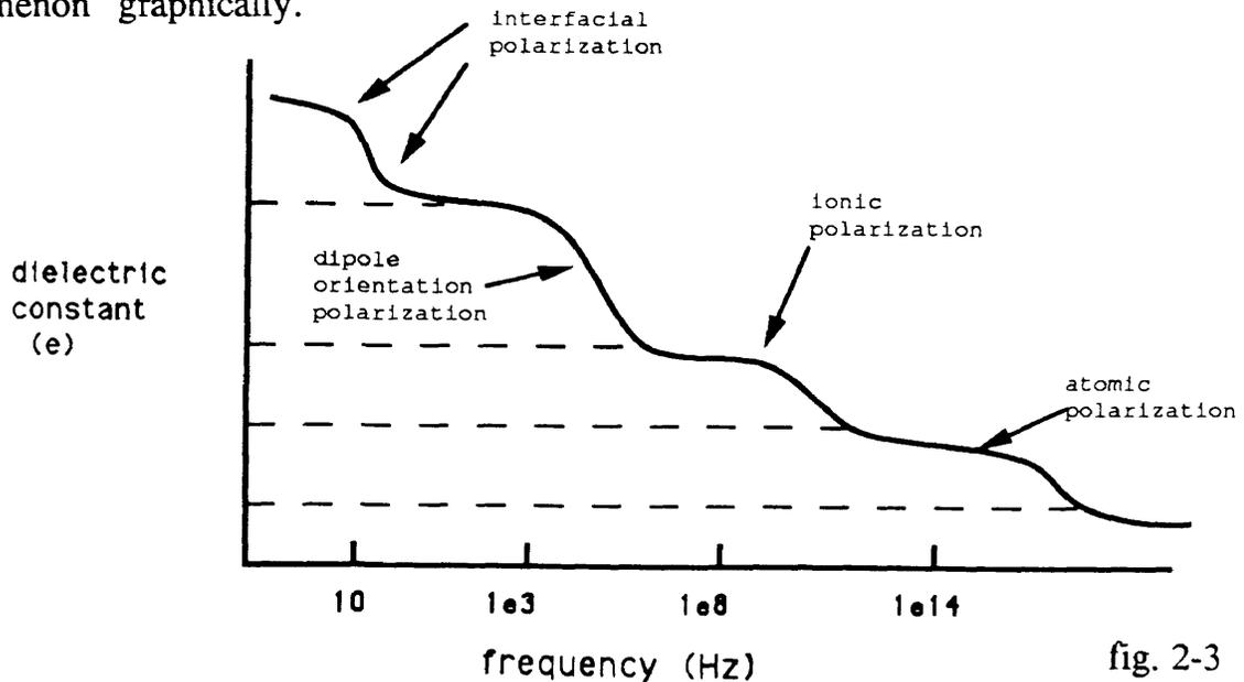
Since  $e = C/C_0$  and  $C_0$  is constant, the drop in  $e$  is analogous to dropping capacitance.
