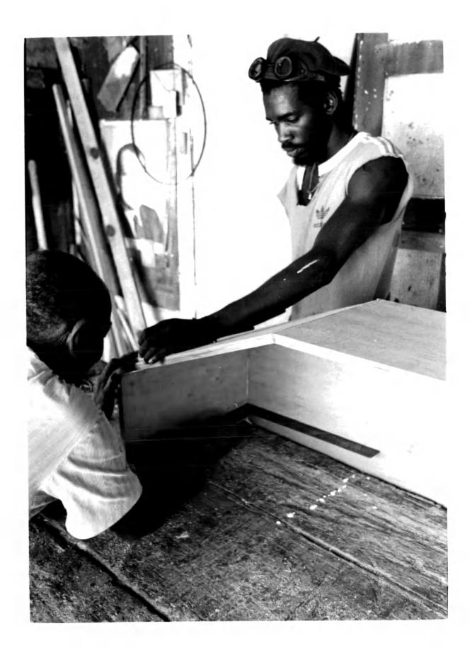
completed, the coffin shelf can be laid on the floor and the long "side" pieces can be brought to the work bench. With a side piece lying on the table, the coffin bottom is brought over it while being held on its side. This allows the coffinmaker to mark where the "breaks" will be located on the side board, exactly in conjunction with the breaks of the coffin bottom. Head and foot marks are only roughly indicated on the side board at this time.
