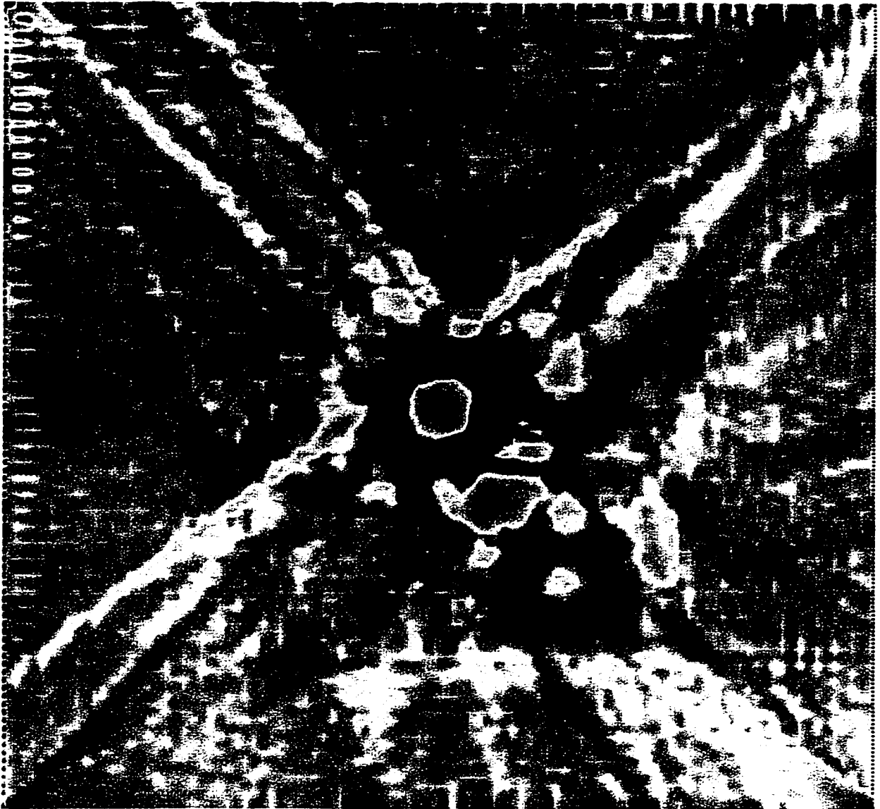
Figure 4.11: Sequential ART reconstruction of two circular flat-bottom holes in aluminum plate. Defect diameters: 29 and 25 mm. Distance between centers: 53 mm. Image size: 200 \times 200 mm. f = 1.2 MHz. Note the level of “salt and pepper noise” throughout the image.
