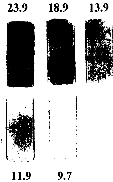
Figure 4-16: Thermal test panel with variations in compaction level. Compaction force is indicated in tons. The thermal image was obtained 50 ms after the heating pulse.
