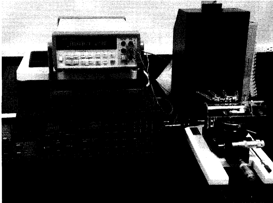
Figure 2.18: Photo of the four-point probe setup utilized at Luna Innovations Incorporated, Advanced Materials Division, Blacksburg, VA. Picture provided via courtesy of Dr. Jonas Gunter.
