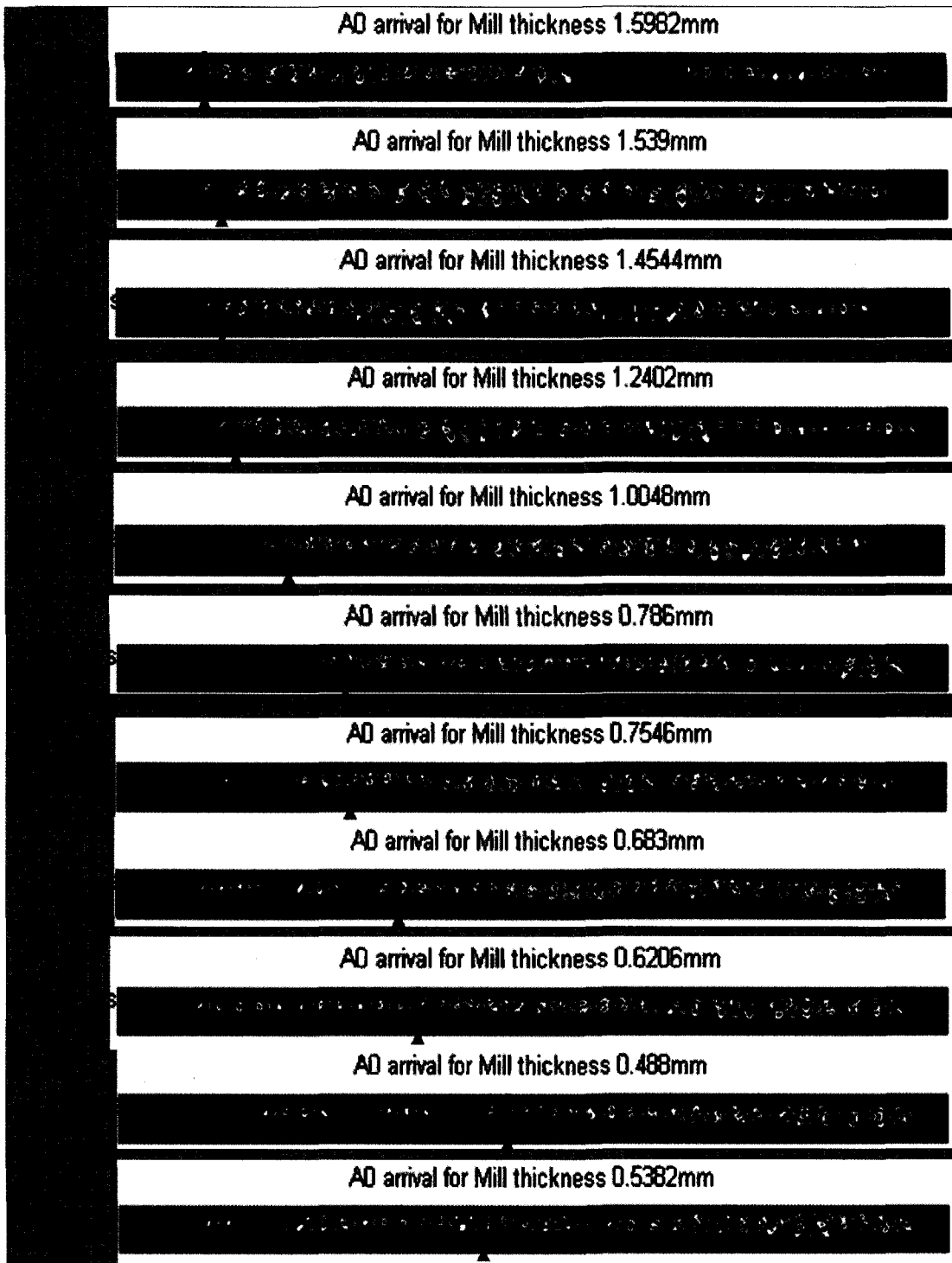
Figure 3.51: Material was removed incrementally from top to bottom with. Fingerprints show the automatically extracted A0 arrival, depicted by the red lines. The arrival time is noted to the left.
