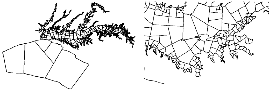
Figure 4.2: Graded MADD based on boundary weights. Left , a model of the Chesapeake bay is decomposed in 1250 subdomains, with weights on all the boundary points and interpolation factor set to zero. Right , detail of the decomposition, the irregular inner polygons represent islands and are part of the initial domain.
