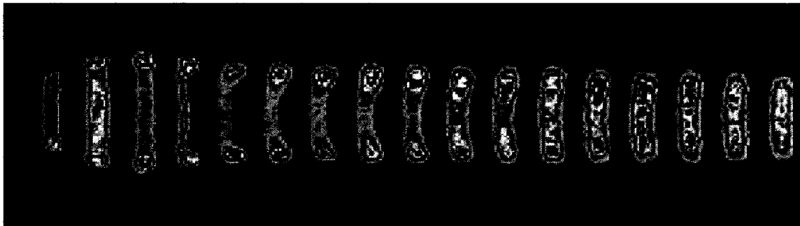
Figure 4.4: Velocity sensitive image. This is a 100-shot average image of Run 69, taken at a delay of 1 \mu s, for a free jet sonic nozzle flow with JPR = 12.8 and Re_{\text{exit}} = 2,685 . The curvature in the lines indicates the difference in velocity between the inner and outer parts of the jet, showing that the jet boundary is moving at a higher velocity than the jet core, particularly in the region just downstream of the Mach disk (which is in the vicinity of the fourth line). Also notice the decrease in curvature further downstream, where viscous effects have had an effect and have reduced the gradient in velocity along a given line.
