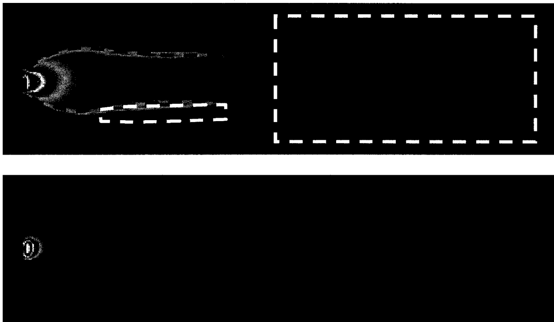
Figure 3.3: Jet core and mixing regions. The black dashed line indicates the approximate boundary of the jet core, in which the mole fraction of nitric oxide, \chi_{\text{NO}} , is nearly constant. White dashed lines indicate mixing regions, where \chi_{\text{NO}} is varying but pressure is nearly constant. The upper image was taken with the laser tuned to the “flow visualization” lines at 226.256 nm. The lower image was taken with the laser tuned to the “pressure-sensitive” lines at 225.693 nm. Both images are the average of 100 uncorrected single-shot images.
