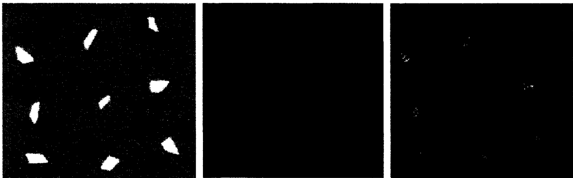
Figure 121: Original low energy x-ray image (left), tungsten subtracted image (middle), and aluminum subtracted image (right) of tungsten foils.
