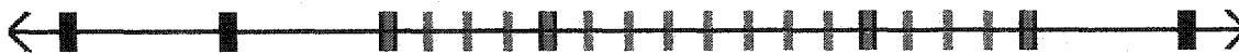
Figure 7.1: This pictorial representation of a one dimensional non-uniform grid contains a refined region where the coarse grid is split into four spatial sub-steps. This refined region would normally be placed around a region of space where large gradients in the field exist.
