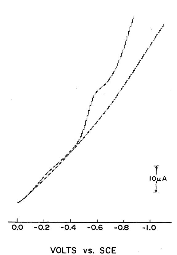
FIGURE 8.Cyclic Voltammogram on Vitreous Carbon Electrode.SCE reference electrode; 16.4  $\mu$ M INT in 50 %ethanol:PBS (v/v); 2 drops Triton X-100 maximasuppressor; scan rates (bottom to top): 10, 50, 100, 200,500, mV/s.
