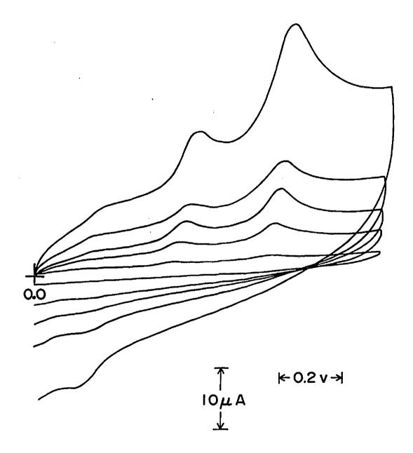
Figure 9.Cyclic Voltammogram on Vitreous Carbon Electrode.SCE reference electrode; 66  $\mu$ M INT in 50 % ethanol: PBS(v/v); 150 mV/s scan rate.
