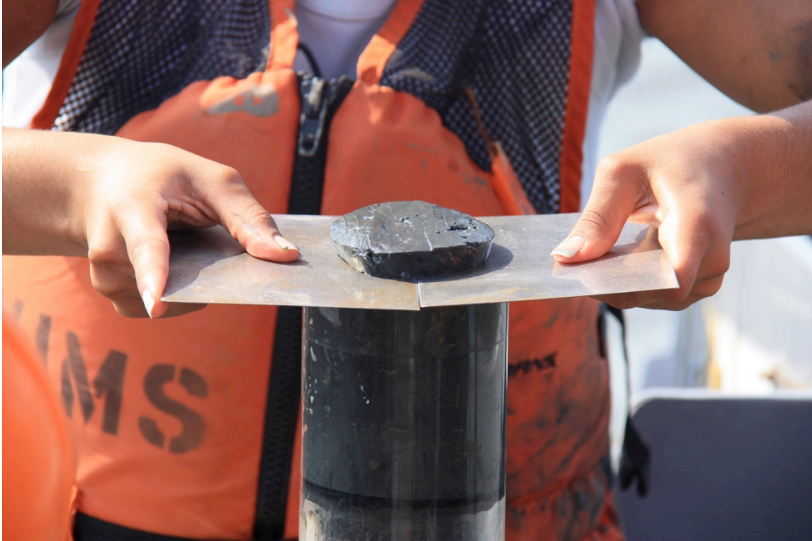
Figure 5. Sediment core extruded and sampled at 1-cm intervals from subcores to be later analyzed at the lab for percentage of total fixed solids (TFS), total volatile solids (TVS), and grain size. Water content (percent moisture) is equal to 100-TFS. TVS is a proxy for percent organic matter
