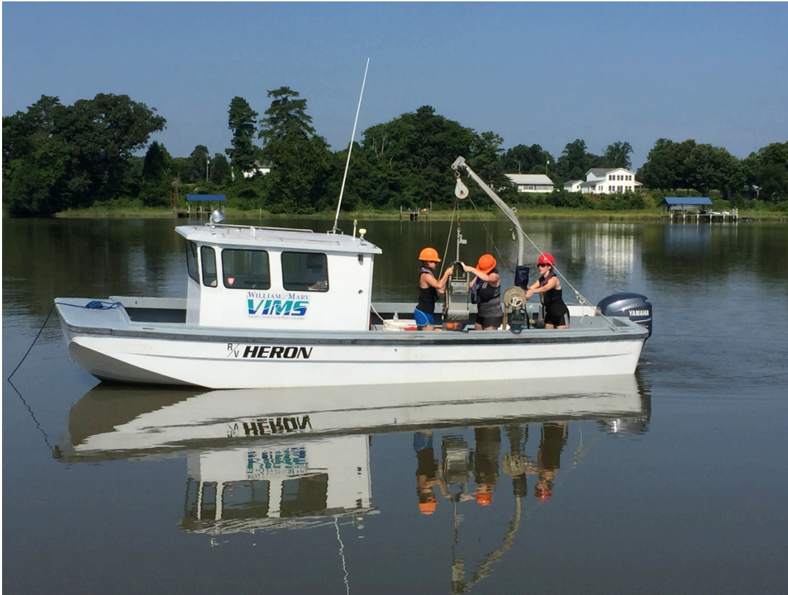
Figure 3. Collection of bottom sediment with GOMEX box-core on board the R/V Heron
