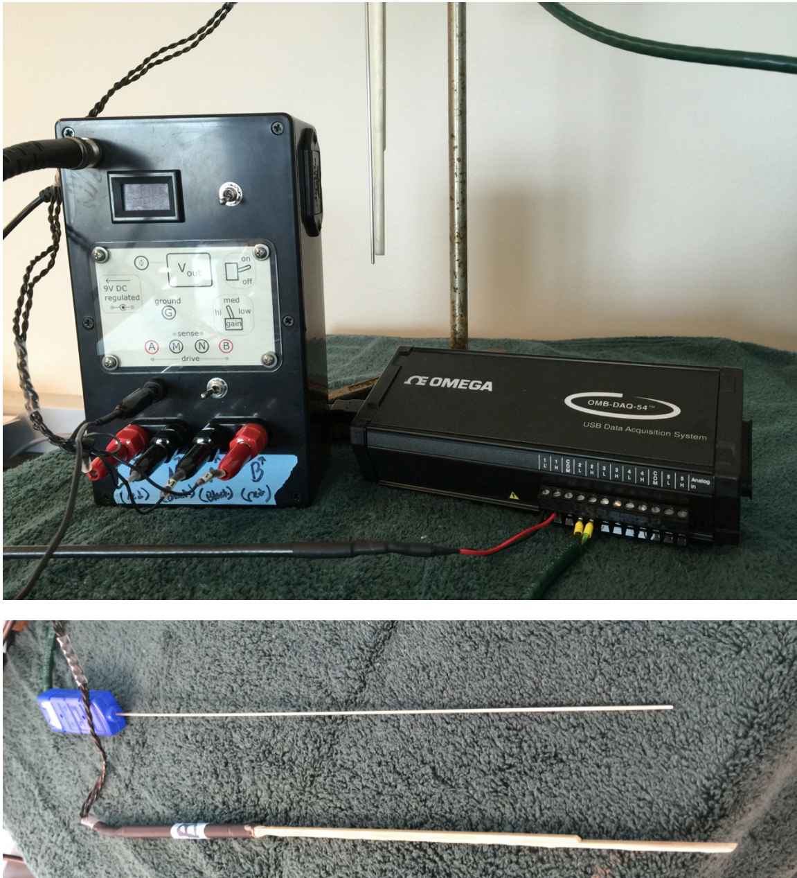
Figure 7. (A) Northwest Metasystems resistivity meter with Omega Data Acquisition System and resistivity and temperature probes (B) Northwest Metasystems resistivity probe and calibrated Omega temperature probe (blue top).
