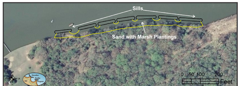
Figure 5-8. Proposed conceptual design planform of the medium sill BMP.
