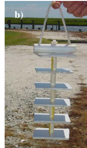
Figure 8. Two types of arrays of ceramic tiles used to assay oyster settlement on reefs.
