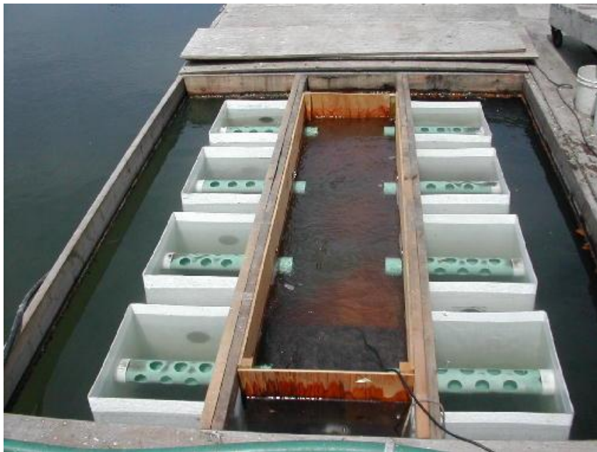
Figure 15 (left): A FLUPSY in the water. A pump pushes water out of the middle trough causing water to be pulled in from the bottom of the silos, past the oysters and back into the trough. (Picture: www.fishersislandoyster.com )
