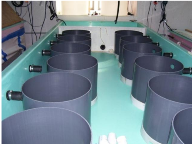
Figure 9 and 10 (above): large scale land upweller systems (figure9: ct-oysters.com) Figure 11 (below): oyster seed in a large scale upwelling system
